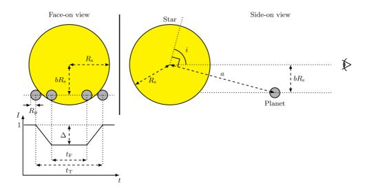
The lightcurve of the normalized intensity, I, as a function of time t is shown in the schematic diagram of the transit above. The average stellar intensity outside the transit is taken as unity. The maximum decrease in the intensity is given by  $\Delta$  in the normalized light curve. For a uniformly bright stellar disk, the radius of the planet,  $R_{\rm p}$ , is related to  $\Delta$  as
