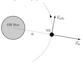
(T07.1) The accretion radius,  $R_{\rm acc}$ , is defined as the maximum distance from the NS at which the stellar wind can be captured by the NS. If the stellar wind speed at the orbital distance of the NS is  $v_{\rm w} = 3.0 \times 10^6 \, \rm m \, s^{-1}$ , find  $R_{\rm acc}$  for the above system in km using standard escape velocity calculations.
