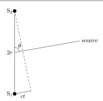
If the direction of the source makes an angle  $\theta$  (see the figure above) with the line joining telescopes  $S_1$  and  $S_2$  we have the path difference  $(\Delta d)$  given as,
