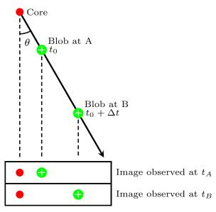
(T05.2) The light emitted by the blob at two different times  $t_0$  (corresponding to position A) and  $t_0 + \Delta t$  (corresponding to position B) reaches the observer at  $t_{\rm A}$  and  $t_{\rm B}$ , respectively. Thus the observed time difference is  $\Delta t_{\rm app} = t_{\rm B} - t_{\rm A}$ .
