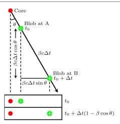
As shown in the sketch above, a signal emitted from the moving blob at B covers a distance  $(\beta c)\Delta t \cos \theta$  less than a signal emitted at A.
